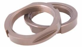
**Lockrings**: An essential part of <u>fixy</u> bikes, the <u>lockring</u> is designed to work with either the Victoire rear hub or any track hub that use the 1.29X24 TPI left thread. Both strong and light, the Victoire <u>lockring</u> is larger than most models available on the market. Made with 7075-T6 alloy, it is 7mm thick, anodized to improve stiffness and can be locked with a lockring wrench or a 36mm wrench.
