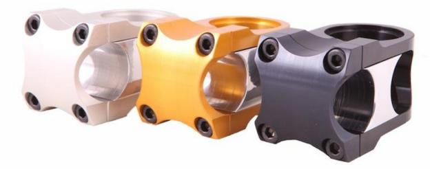
**Stems**: Dedicated to the art of Bike Polo, the S-42 stem is machined from <u>solid block</u>, 7075-T6 alloy and uses an innovative clamping system for easy installation. Also, weighing in at 4.8 <u>oz</u>, this stem is half the weight of a classic BMX stem and a short length (42 mm) for maximum maneuverability and control. Finally, eliminating the back bolt helps riders avoid knee injuries while in the field.
